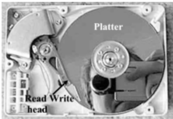
The inside of a hard disk displaying the read/write head traveling over the platters.
